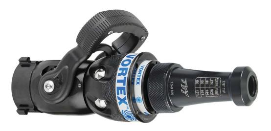
The TFT VORTEX enhances the use of a smooth bore nozzle. With just a simple twist, the VORTEX moves from a hard hitting straight stream to a uniformly dispersed pattern without gating the valve and reducing the fire flow. Available in a tip only, with valve or with valve and grip. A complete range of smooth bore tips are offered separately.
